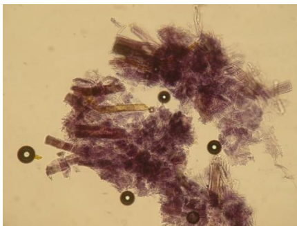
Fig. 10 Blue colour by Chlor zink iodine on a pine tree fibre with Tüpfel, yellow a wood fibre of unidentified sort, 200x, Meh. 5046, 17th cent.
