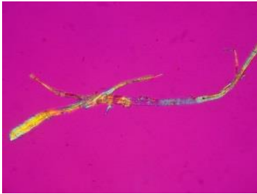
Fig. 4 Linen fibres 200x middle lamdaplates OW position: indigo taken from codex Meh.7954 page 8, 1483
