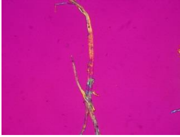
Fig. 3 Linen fibres 200x middle lamdaplates NS position: orange taken from codex Meh.7954 page 8, 1483
