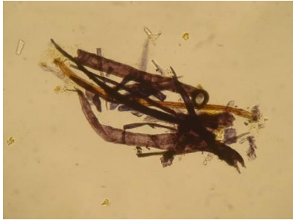
Fig. 10 Blue colour by Chlor zink iodine on a pine tree fibre with Tüpfel, yellow a wood fibre of unidentified sort, 200x, Meh. 5046, 17th cent.
